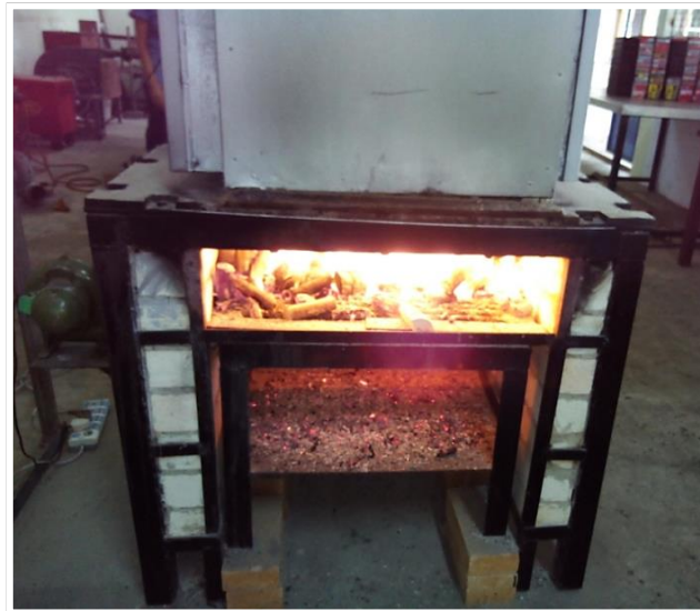
Figure 3: Biomass combustion unit located underneath the heat exchanger unit
