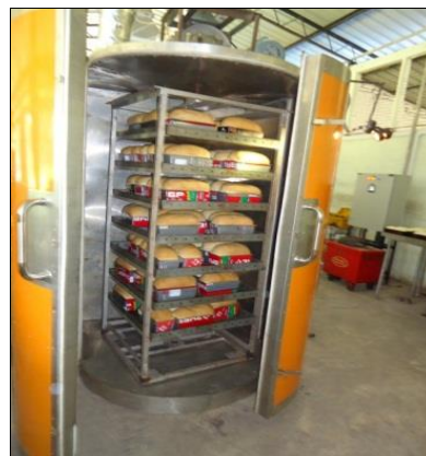
Figure 8: Rotating trolley is mounted permanently inside the oven chamber
